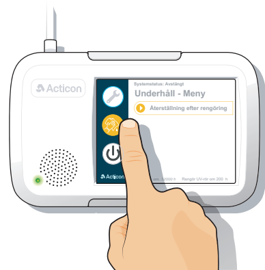
Figure 9 - Press "Reset after cleaning"
