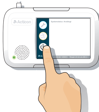
Figure 16 - Press "on/off" and the system starts
