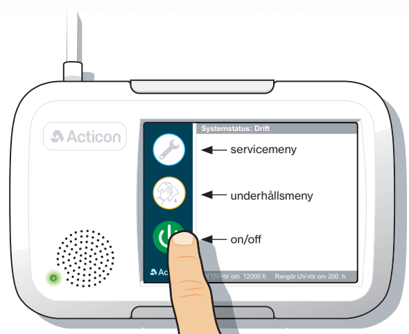
Figure 2 - The top of the screen shows whether the system is running or off. At the bottom, it shows when it's time to replace the UV tubes and clean the system. The cleaning interval can be changed in the service menu
