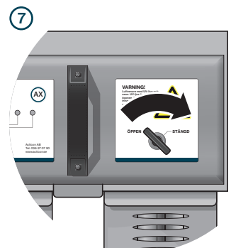
Lock. The system cannot start if the door is not locked.
